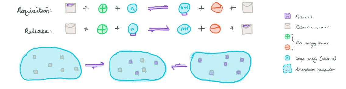
An example passive scheme analogous to the supply of amino acids (purple floppies) in cells by tRNA carriers (grey cases). Plus and minus tokens correspond to a source of free energy driving computation, shown here by the transition from state n to n+1. Meanwhile, the resource pool is entropically driven towards a state of half-full.
